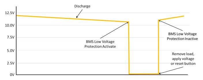
The discharge curve below is a 20Hr test on a LiFePO<sub>4</sub> battery. You can see that less than 5% of the battery's overall capacity is delivered between 12.0V and the voltage cutoff.
