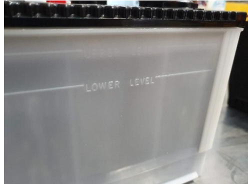
Figure 1 Electrolyte levels in a battery
