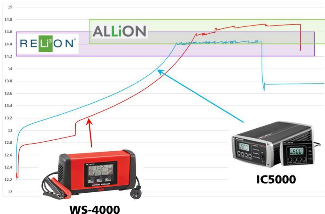
**When selling a lithium battery, it is important that you discuss battery charging with the Customer. In most instances using a lead acid charger set to AGM will work fine however explaining the voltage limits will help them understand what is required. Providing them with a copy of the Product Data Sheet for the battery they have purchased is a good way to ensure the Customer is aware of the battery specifications for charging and discharging.**
