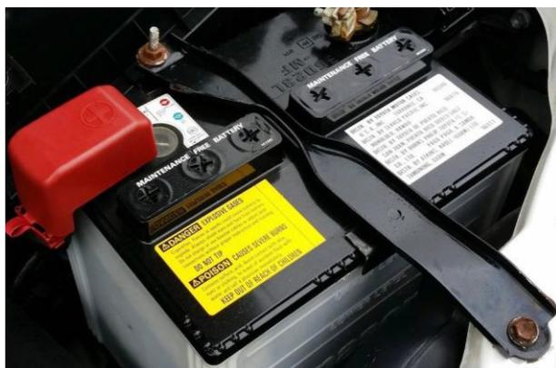
Hold down clamps are designed to retain the battery and prevent it from moving or vibrating. When it comes to the top hold down clamp, you need to keep in mind that you are retaining a plastic case. Excess force will deform the case, potentially damaging the lid to case joint. This will result in battery acid leaking from the case and damaging the vehicle.
