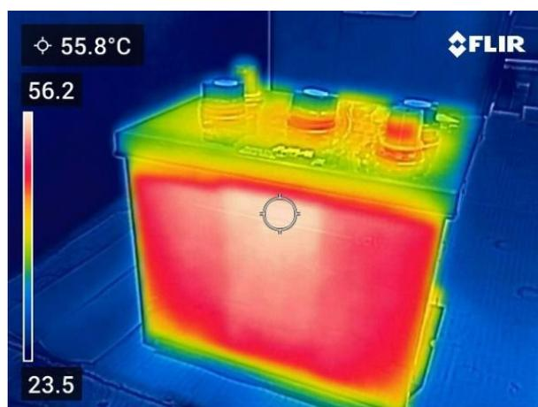
The second image (above right) was taken at 12:30pm. This is now two hours after the batteries were filled. The maximum temperature recorded had increased to just over 56°C.
